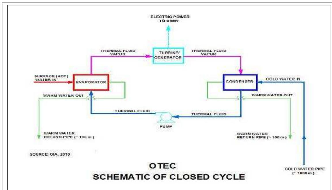
*Figure 1. Schematic of an OTEC closed-cycle system with ammonia as working fluid.*
